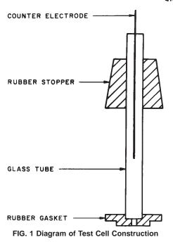
3.2 *Cell* (Fig. 1) for containing the electrolyte during test. It may be constructed from the following components:<sup>4</sup>
