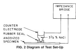
desirable to modify this apparatus so that larger areas can be measured. Because this area may vary owing to variations in cell gasket size and wear during use, the cell should be standardized daily.
